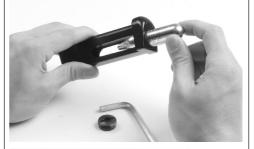
Tighten the piercing knob by turning it clockwise until you hear a hissing sound indicating the CO2 cartridge has been pierced. Tighten an additional quarter rotation
